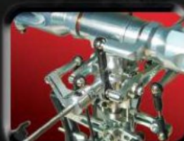
CNC cyclic control arms and hiller assembly
